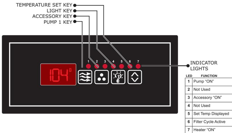
**Default System Operation:** When power is applied, or there is a temporary loss of power, the system will initiate its default programming. The filter cycle will begin 24-hours after the system has been powered up. The filtration cycle will be active for 1-hour and will repeat every 24-hours. The temperature will be maintained at 100°F.
